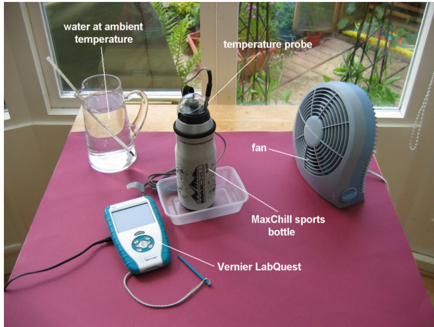
Figure 1 Setup of MaxChill™ sports bottle with Vernier LabQuest to investigate evaporative cooling
