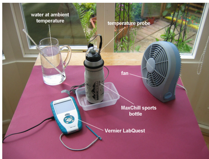
Figure 4 Setup of LabQuest with the temperature probe and the MaxChill™ sports bottle
