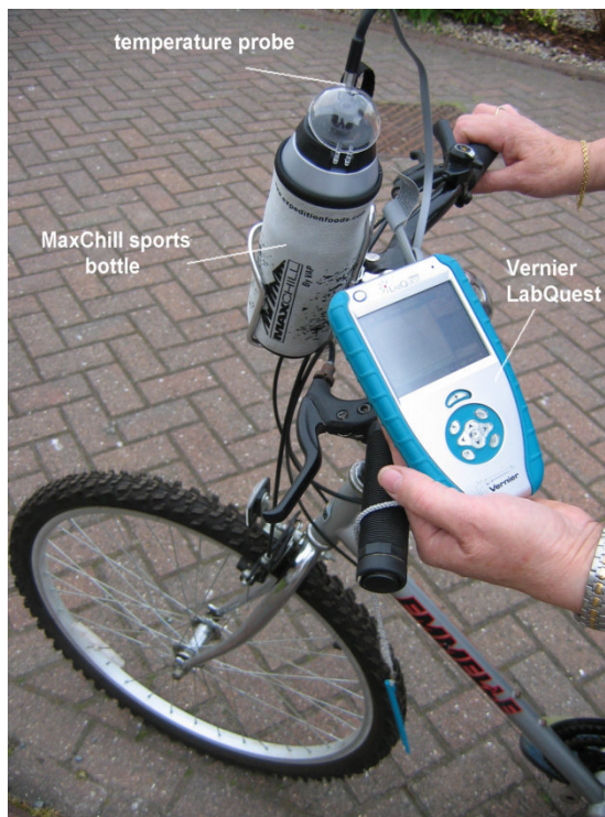
Figure 1 Sensing the temperature of a MaxChill™ sports bottle with LabQuest
