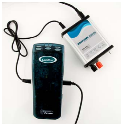
Power Amplifier connected via the BTA cable to CH 4 of a LabPro
