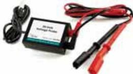
The 30-Volt Voltage Probe is used to measure electrical potentials in the range of -30 to +30 volts. This sensor uses an internal voltage divider connected to the +/-10 volt input of the interface. Use this sensor in experiments that involve voltages larger than 10 volts, such as when working with large solar panels.
